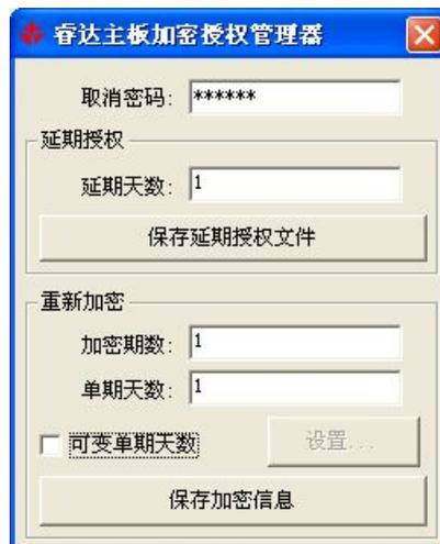
Re-encryption process is exactly the same as the encryption process, but only need to input the cancel password and no need to connect the control card.
