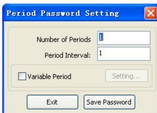
The period password function can be used for use management, such as installment, product on trial, the distributor payment and so on. It can be at most used for 20 encrypted phases. Generally, the limit days of single-use are less than 200 days. When expiration, the controller will lock the machine automatically, user cannot use the machine for processing normally.
