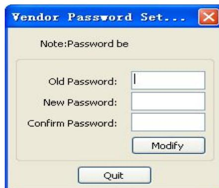
Enter the old password, the new password and re-enter the new password at the “Confirm Password”, then click the "Modify" button to complete the vendor password settings.
